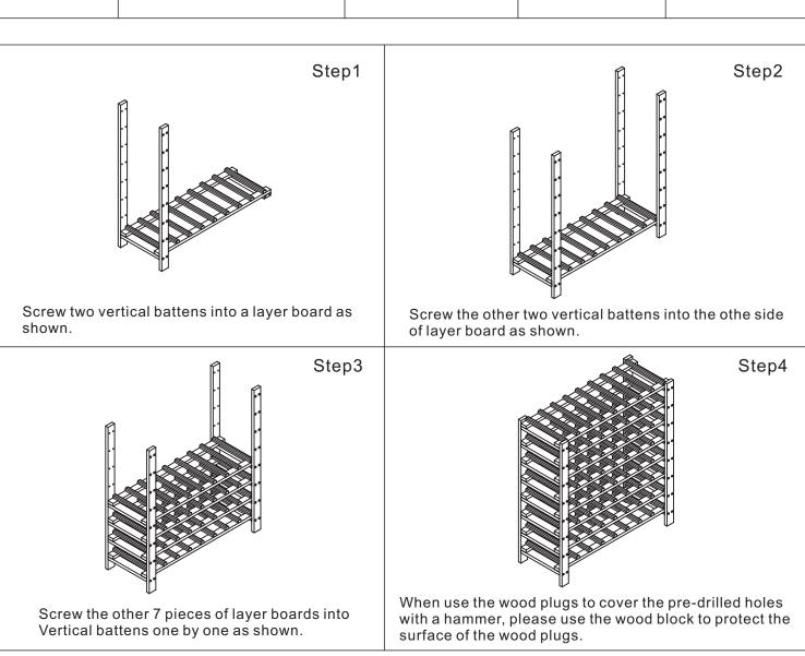
Important: The wood plugs are used to cover the screw holes.
